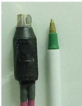
Figure 7. Picture of MOXTEK low-power tube.
