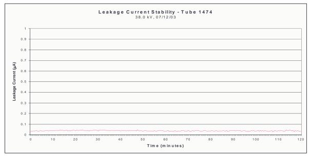
Figure 7. Typical leakage-current stability test
