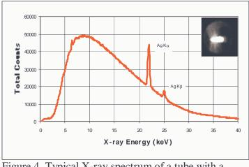
Figure 4. Typical X-ray spectrum of a tube with a collimator and near-centered beam spot (insert)
