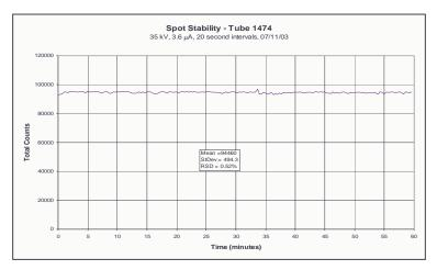
Figure 5. Typical graph of the X-ray detector total number of counts vs. time for a stable tube run at 35 KV and 3.5  $\mu$ A
