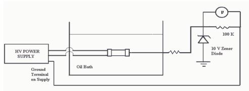
Fig. 6. Electrical circuit to measure leakage current
