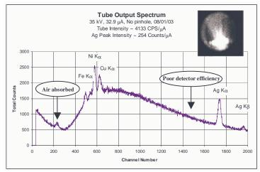
Figure 3. Typical X-ray spectrum of a tube with no collimator and near-edged beam spot (insert)
