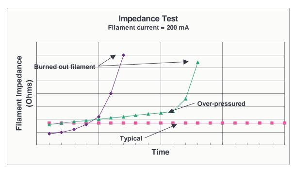
Figure 8. Three typical filament-impedance behaviors a tube filament can undergo
