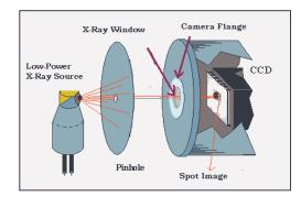
Figure 1. Pinhole-CCD camera concept for taking X-ray images
