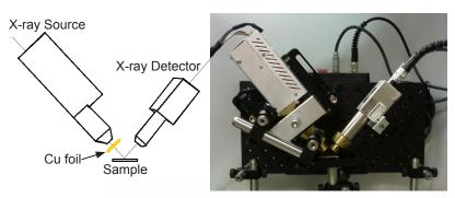
Figure 1. On the left is a sketch of the XRF setup, outlining the most critical parts. On the right is an image of the set up where all the components including collimators can be seen.
