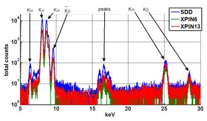
Figure 3. XRF Spectra collected from a naval brass sample, over 30 seconds, with all the major peaks labeled. Y axis of counts is in a log scale.
