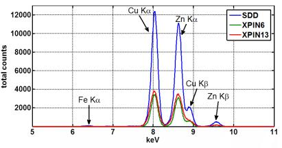
Figure 4. The same XRF Spectra collected in Figure 3, with a linear y-scale and energy range from 5 to 11keV.
