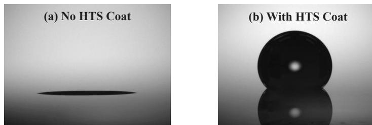
Figure 1. Demonstrates the hydrophobic properties of the HTS protective coating on a wire-grid polarizer. (a) is not treated, showing a flat drop of water. (b) Is treated with hydrophobic HTS coat, showing a droplet of water with high contact angle.
