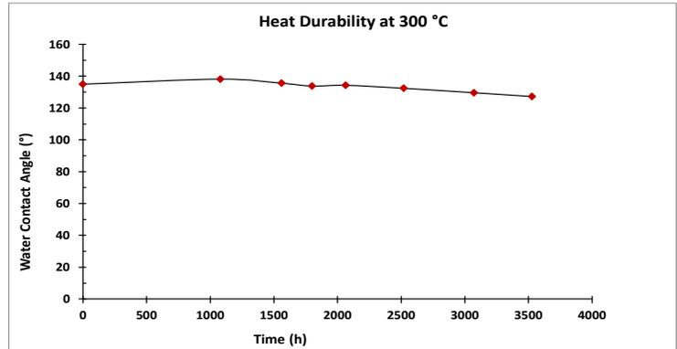
Figure 3. The heat durability of the HTS coated polarizer was demonstrated by plotting the water contact angle during exposure to 300°C. Parts maintained a WCA > 120° for over 3,500 hours.
