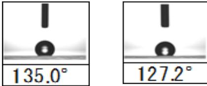
Figure 2. Images above show water droplet on wire-grid polarizer. Water contact angle was measured before and after 300°C exposure for over 3,500 hours.
