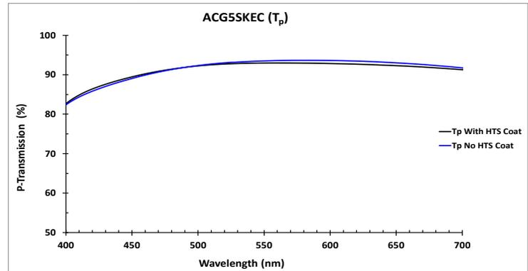
Figure 4. Minimal Tp Performance Impact of HTS Coat.
