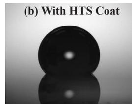
Figure 1. Demonstrates the impact of the HTS protective coating on a wire-grid polarizer. (a) is not treated, showing a flat drop of water. (b) Is treated with hydrophobic HTS coat, showing a droplet of water with high contact angle.
