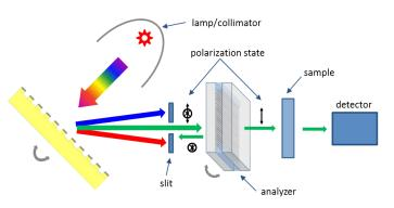
Figure 1 Simplified spectrophotometer with analyzer
