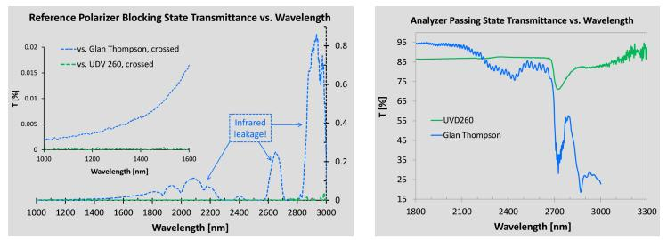
Figure 3 Infrared performance comparison of UVD260 and calcite Glan-Thompson analyzers. (a) Blocking state transmittance measurements of the same reference polarizer using GTh (----) and UVD260 (----) analyzers. Inset shows magnified scale away from absorption resonances. (b) GTh (---) and UVD260 (----) passing state transmittance.
