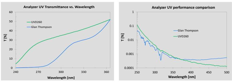
Figure 2 Performance comparison of ProFlux UVD260 and Glan-Thompson polarizers in an analyzer application. (a) Analyzer passing state UV transmittance comparison. (b) Reference part measurement
