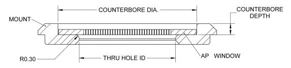
Figure 5 Geometry Requirements for Window Counterbore
