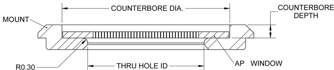
Figure 5 Geometry Requirements for Window Counterbore
