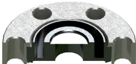
Figure 1 Typical Assembly of Beryllium Window
