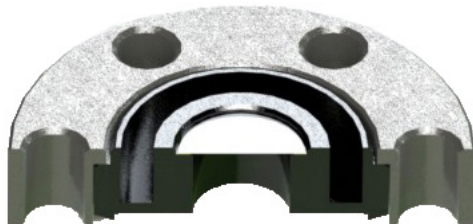
Figure 1 Typical Assembly of Beryllium Window
