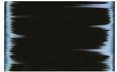
Figure 2: To avoid this type of wicking damage always use gloves.
