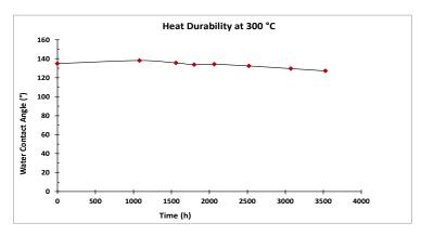
Figure 3. The heat durability of the HTS coated polarizer was demonstrated by plotting the water contact angle during exposure to  $300^{\circ}$ C. Parts maintained a WCA >  $120^{\circ}$  for over 3,500 hours.
