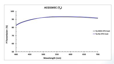
Figure 4. Minimal Tp Performance Impact of HTS Coat.
