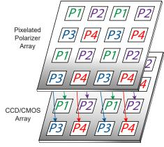
Pixelated polarizer aligned to camera array.
