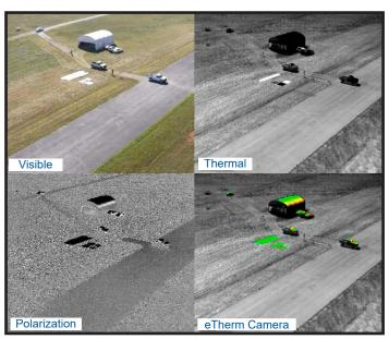
Visible, Thermal, Polarization and processed eTherm images showing different data products in a target identification application.
