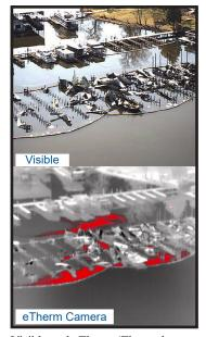
Visible and eTherm (Thermal + Polarization) images identifying oil spill after a marina fire near Huntsville, AL.
