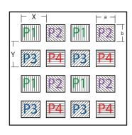
Typical layout of a 4-state pixelated polarizer array.
