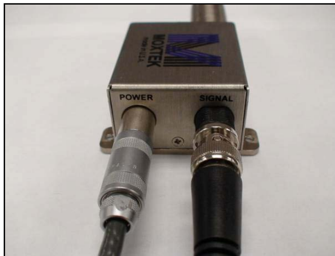
Figure 6 Power and Signal Cable Attached
