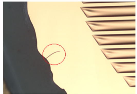
Figure 8 Wrinkle in film that is not more than half way across the flange, acceptable.
